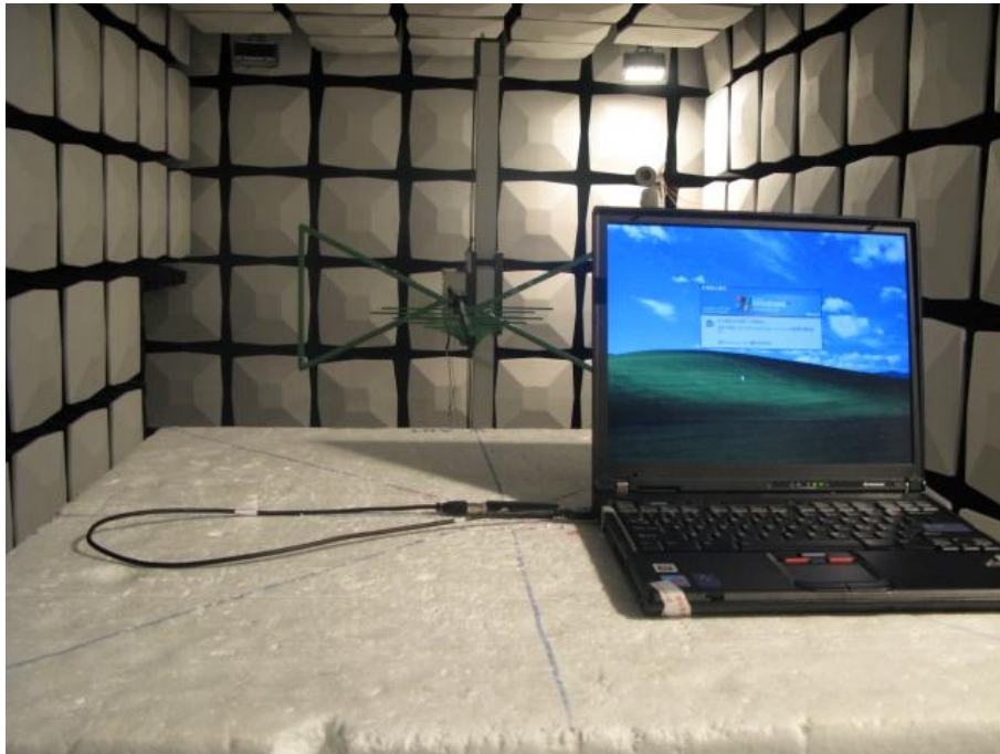
Radiated Spurious Emission (below 2GHz)
