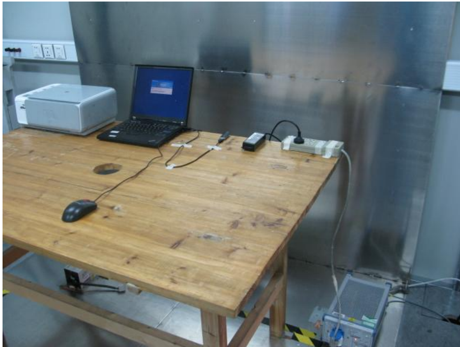
Conducted Emissions for AC Power
