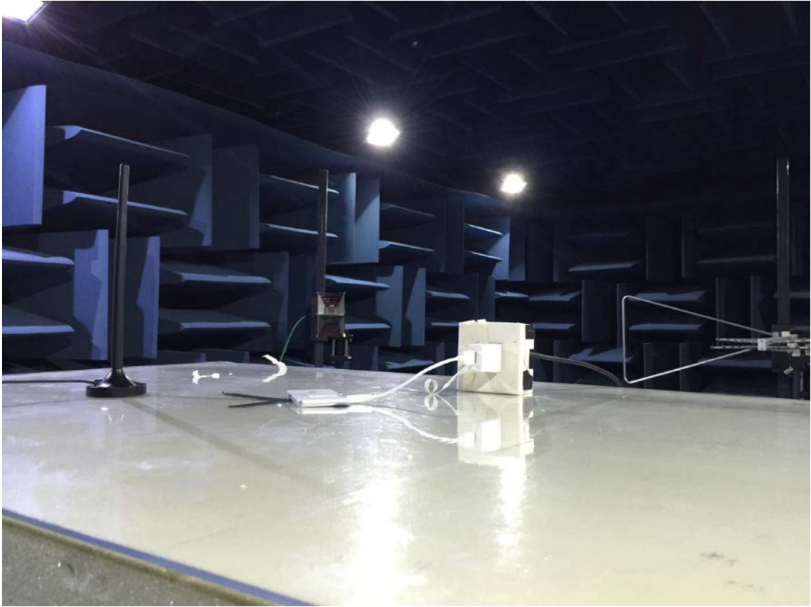
Radiated Spurious Emission (3GHz to18GHz)
