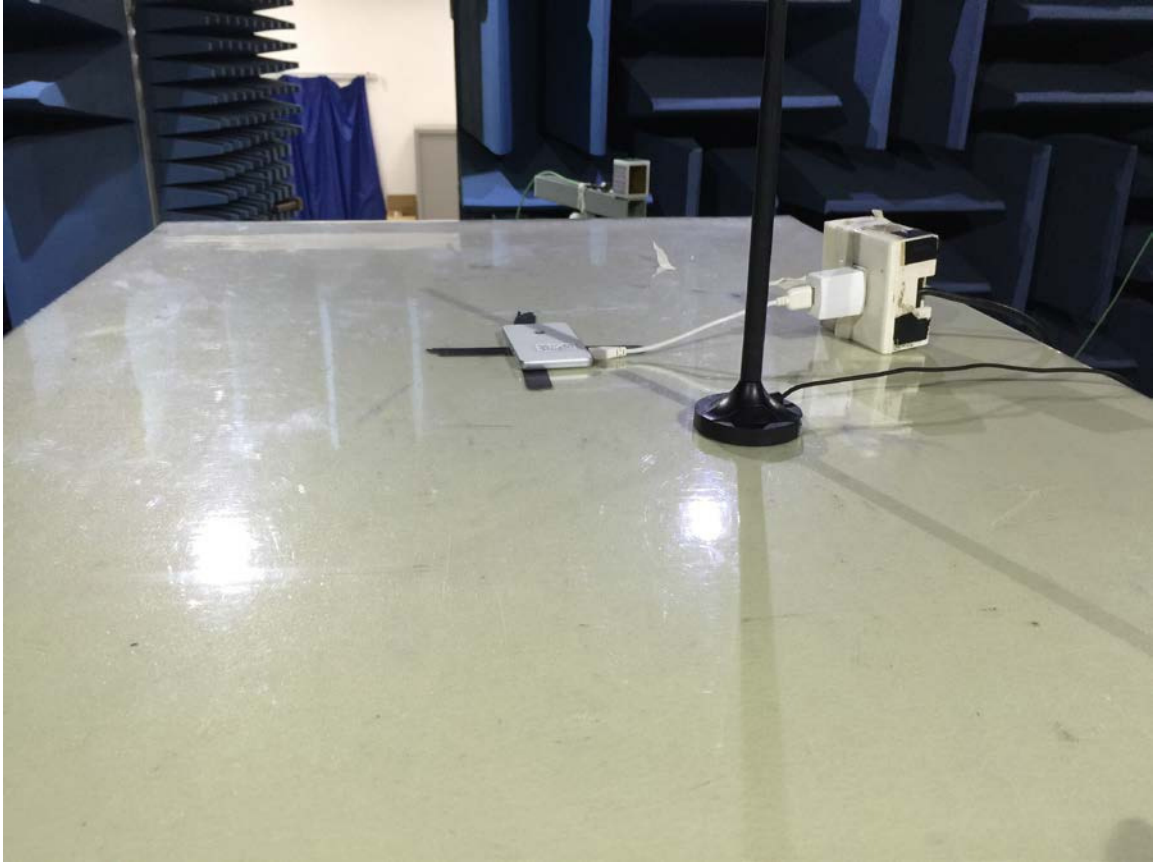
Radiated Spurious Emission (18GHz to26.5GHz)
