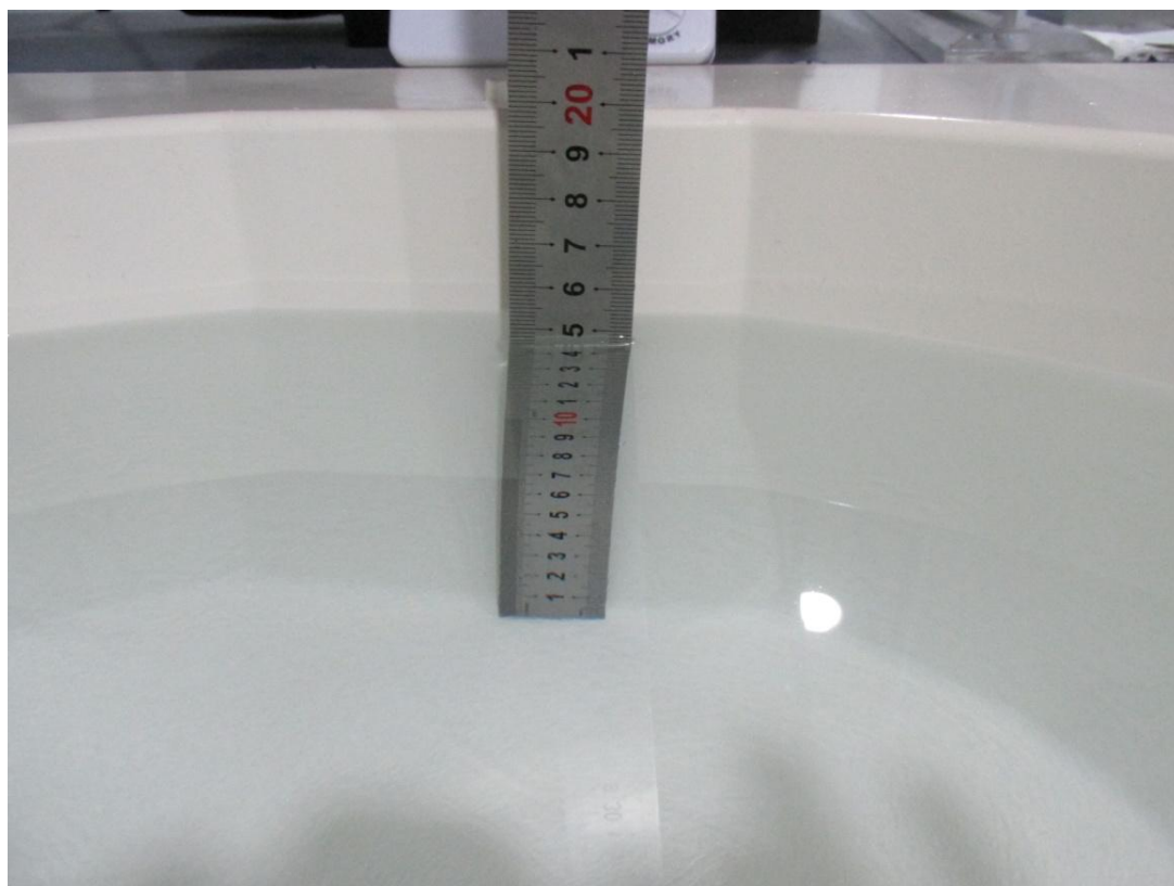
Fig.8 Body Liquid of 835MHz(15cm)
