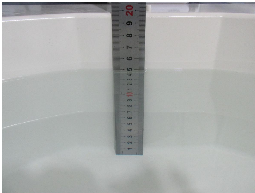
Fig.10 Body Liquid of 1900MHz(15cm)
