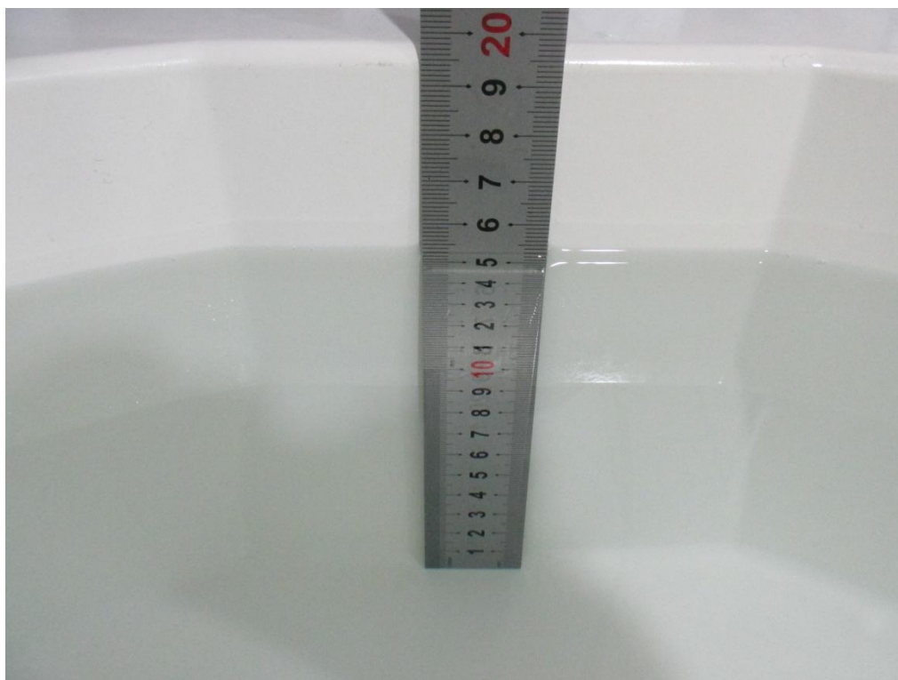
Fig.11 Body Liquid of 2450MHz(15cm)
