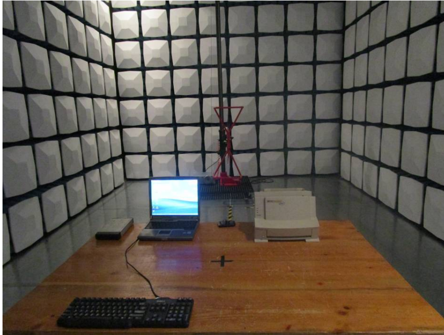
Radiated Emission Below 1GHz Front View (Downloading Mode)
