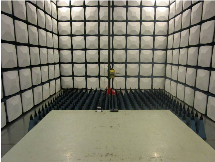
Radiated Emission Above 1GHz Front View (Charging Mode)
