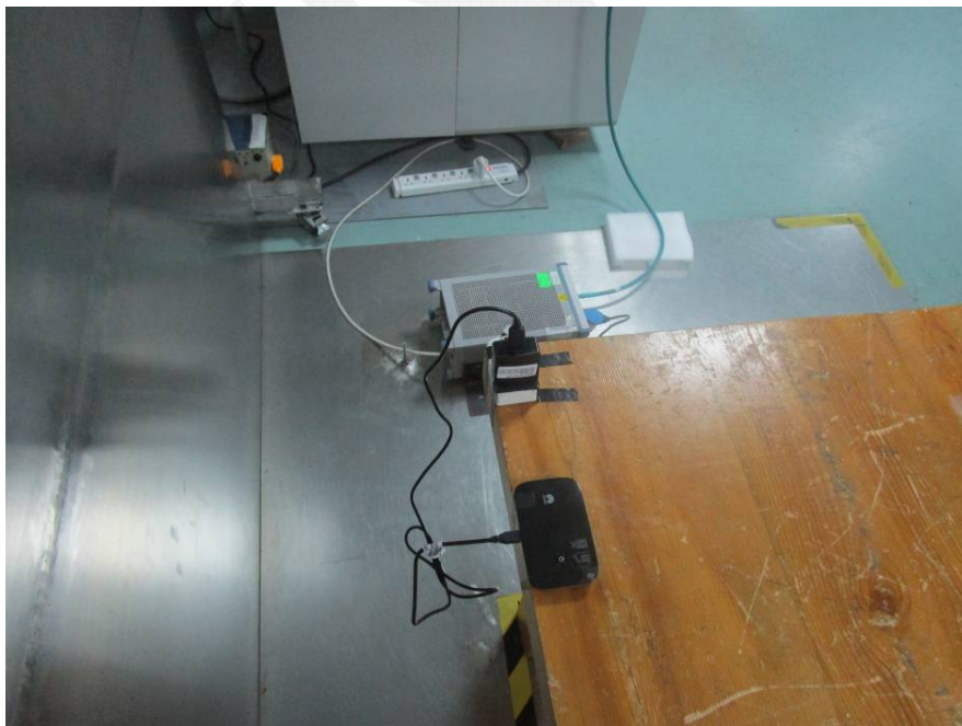
Conducted Emissions – Side View (Charging Mode)
