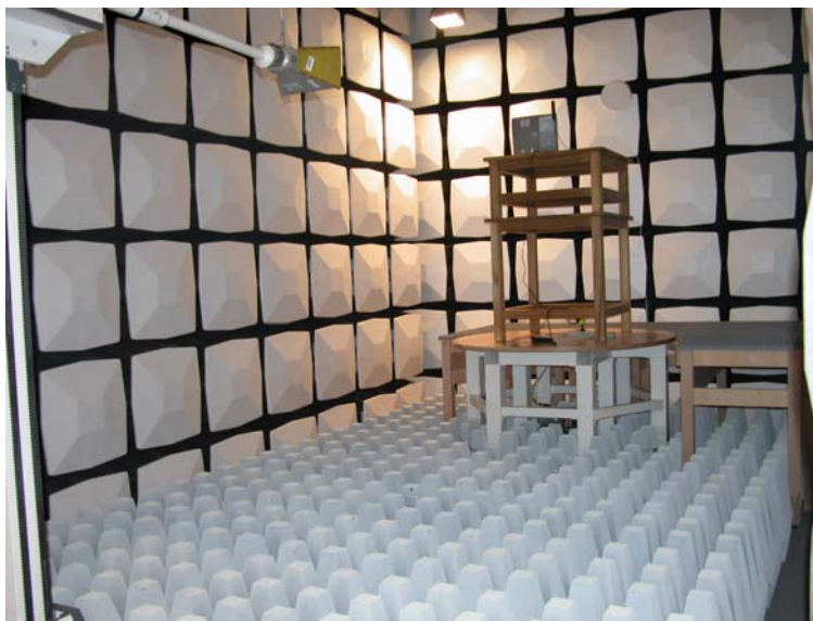
Radiated Spurious Emission (above 1 GHz , with external antenna)
