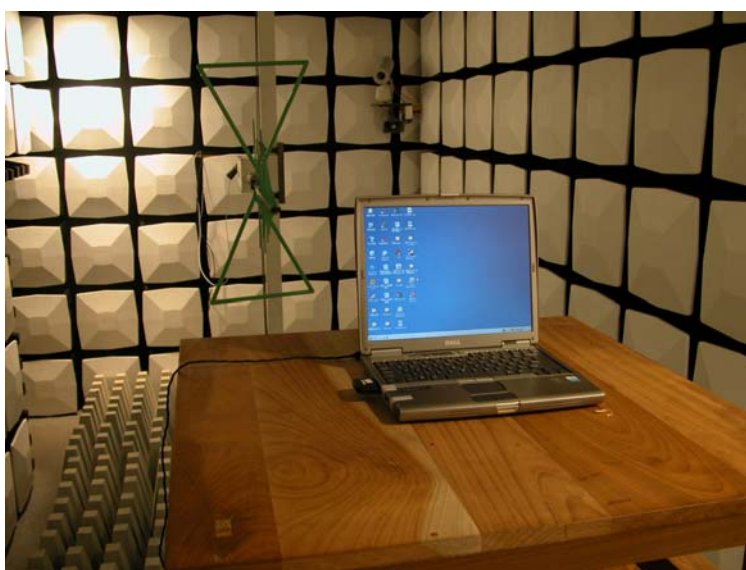
Radiated Spurious Emission (bellow 1 GHz , without external antenna)
