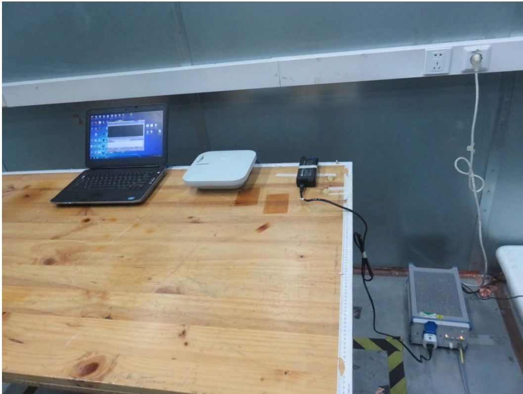
Picture 3 Conducted Emission Test Setup
