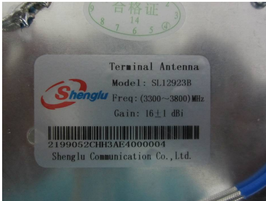
EUT – LTE Antenna Label View
