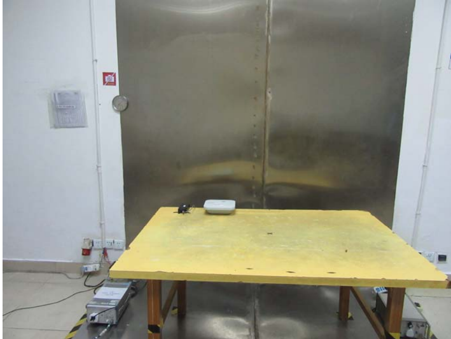
Conducted Emissions – Front View
