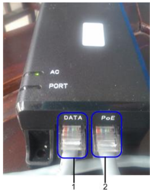
Figure 3-16 Connecting the PoE adapter
