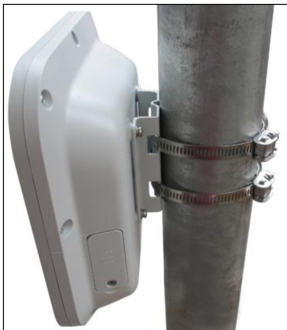
Figure 3-6 The installation is complete
