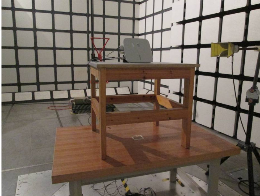
Transmitting Radiated Emissions (Below 1 GHz)
