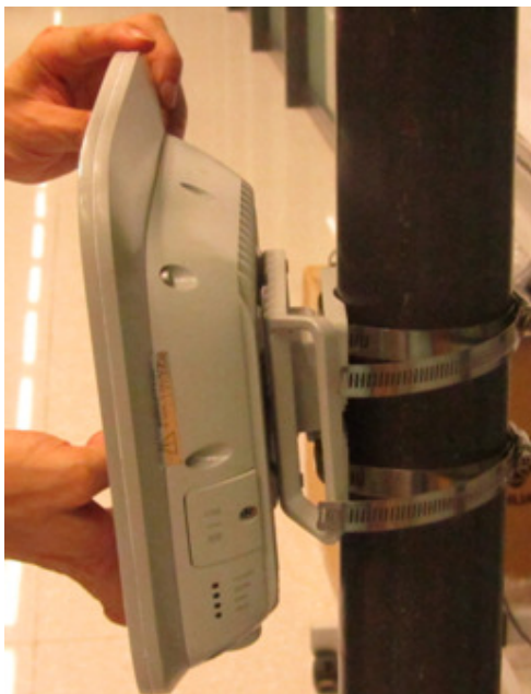
Figure 3-7 Installing the eA660 on the wall-mounting frame
