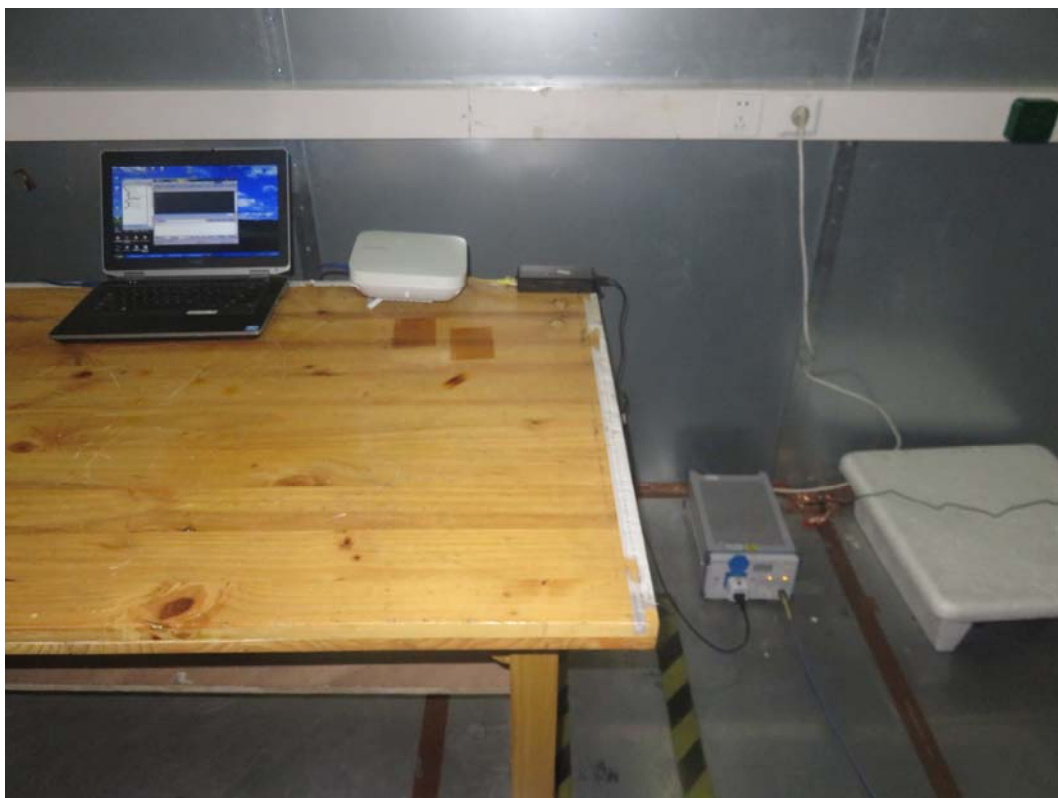
Picture 3 Conducted Emission Test Setup
