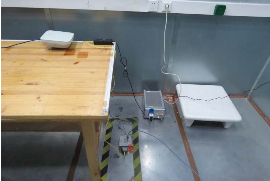
Picture 3 Conducted Emission Test Setup
