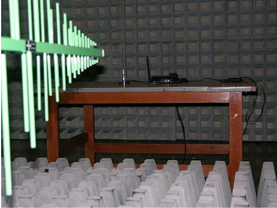
Radiated Spurious Emission (below 1GHz)
