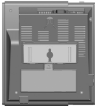
Figure 4-8 Wall-mounting bracket installation
