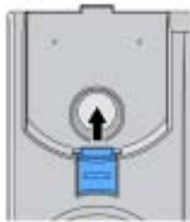
Figure 4-7 Handset retaining clip installation
