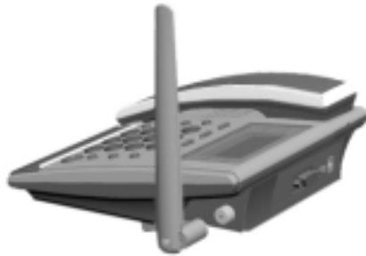
Figure 4-6 Installing an indoor antenna for the FWT
