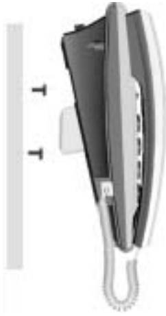
Figure 4-9 FWT vertical placement
