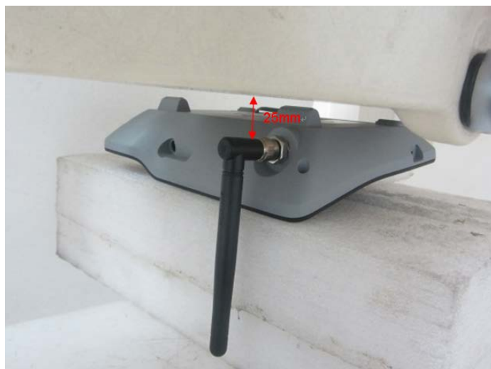
Photo 7: Back side- antenna vertical (25mm)
