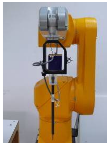
Figure 3. ES3DV3 E-field probe
