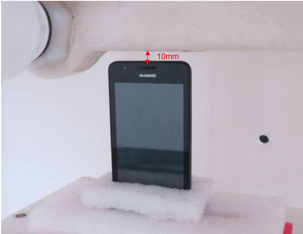
Picture 17: Top Edge, the distance from handset to the bottom of the Phantom is 10mm
