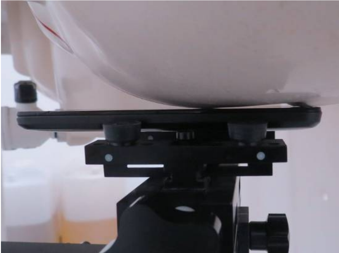
Picture 9: Left Hand Touch Cheek Position
