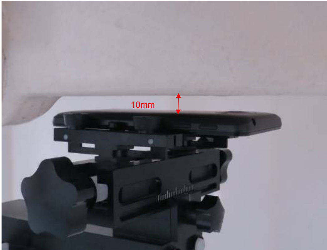
Picture 13: Back Side, the distance from handset to the bottom of the Phantom is 10mm
