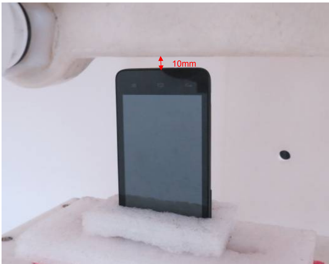
Picture 18: Bottom Edge, the distance from handset to the bottom of the Phantom is 10mm
