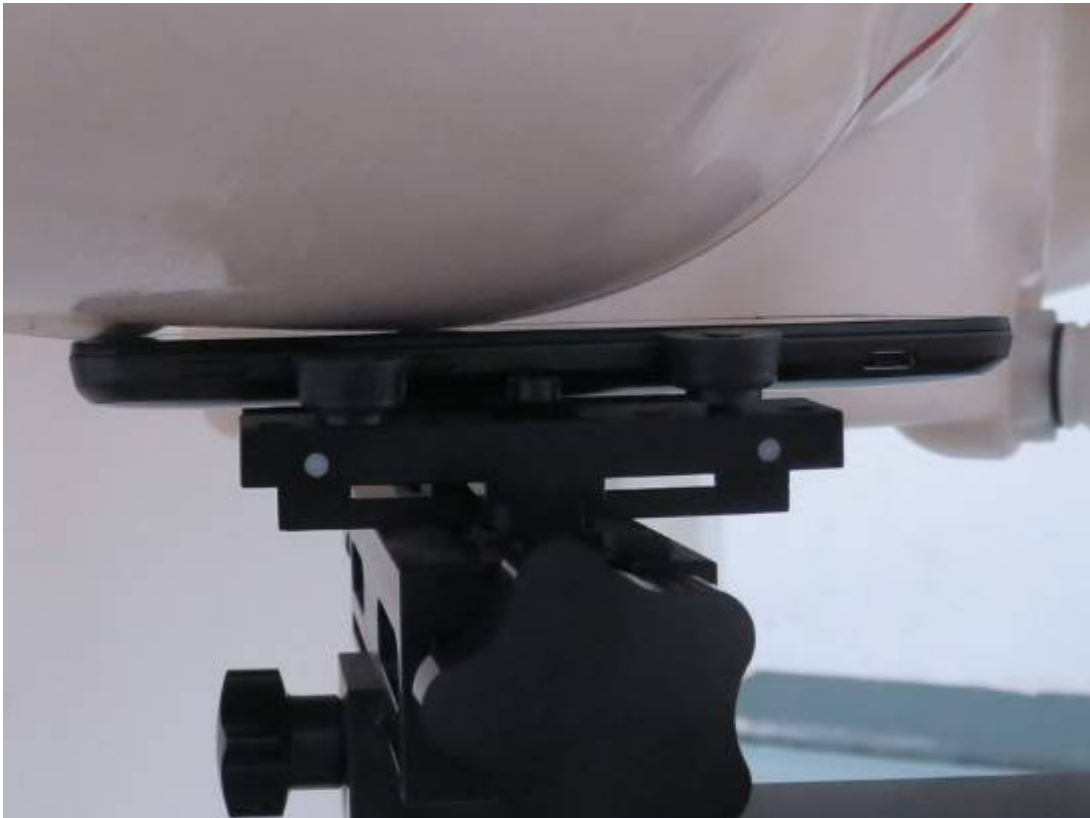
Picture 11: Right Hand Touch Cheek Position
