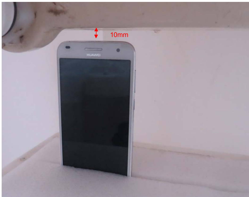
Picture 21: Top Edge, the distance from handset to the bottom of the Phantom is 10mm
