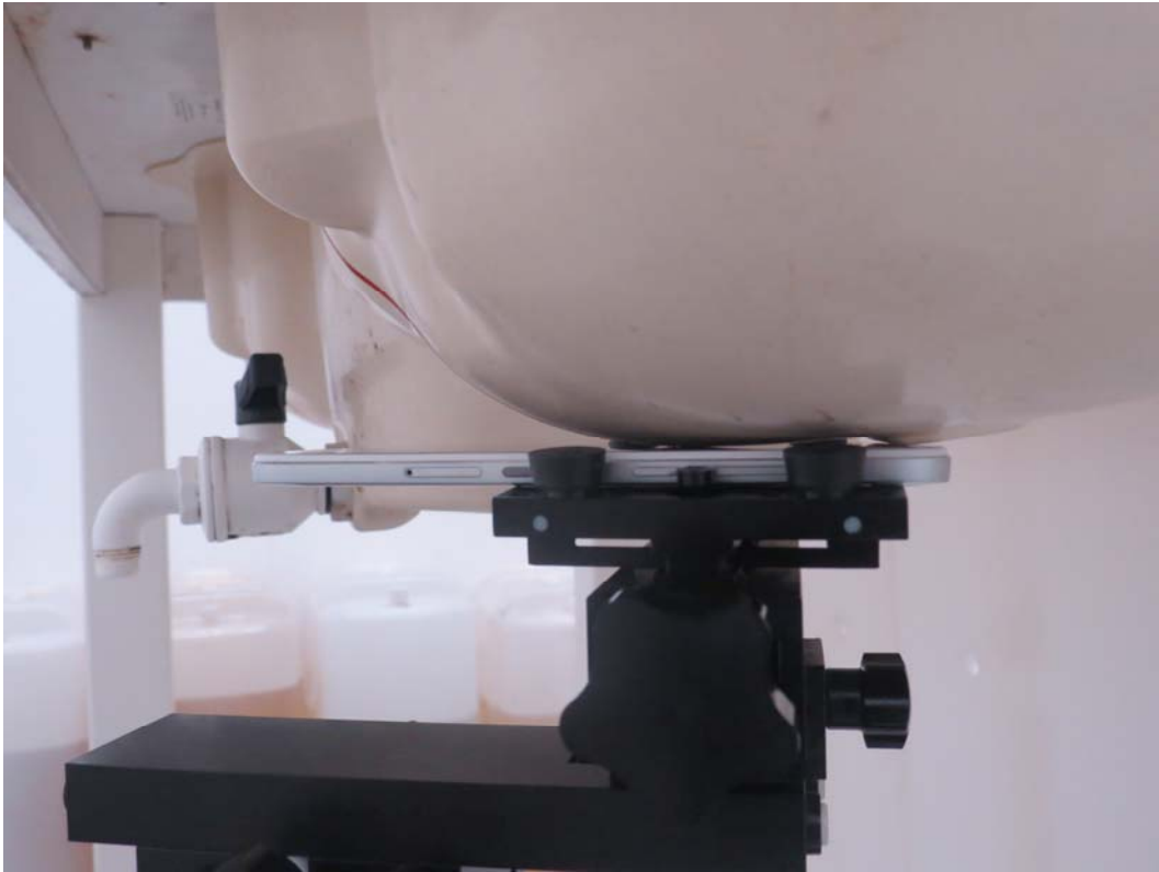
Picture 11: Left Hand Touch Cheek Position
