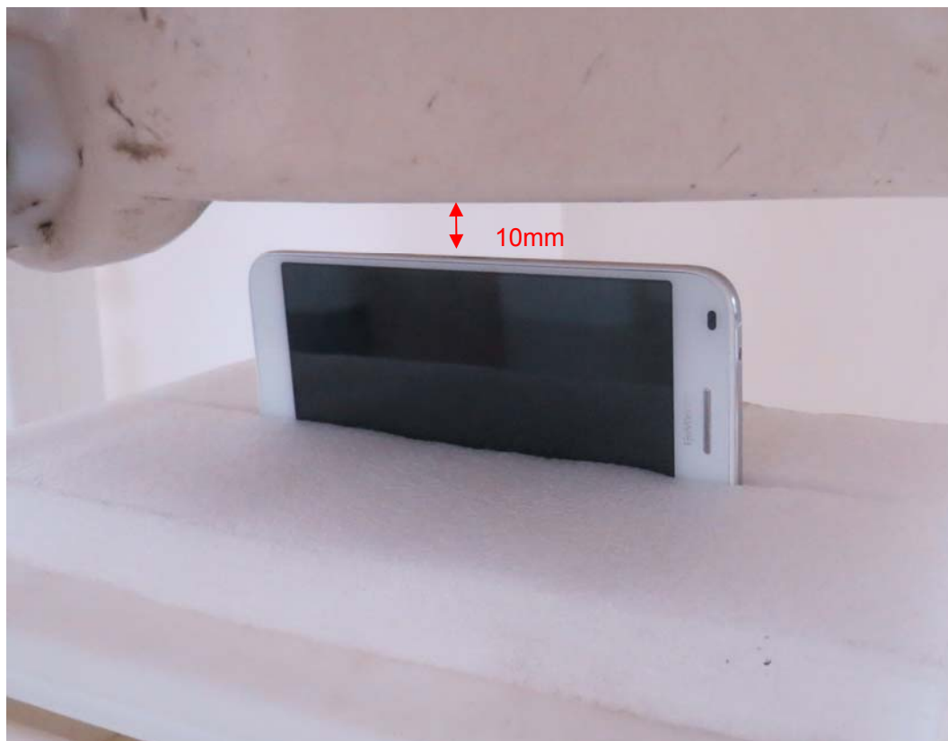
Picture 19: Left Edge, the distance from handset to the bottom of the Phantom is 10mm
