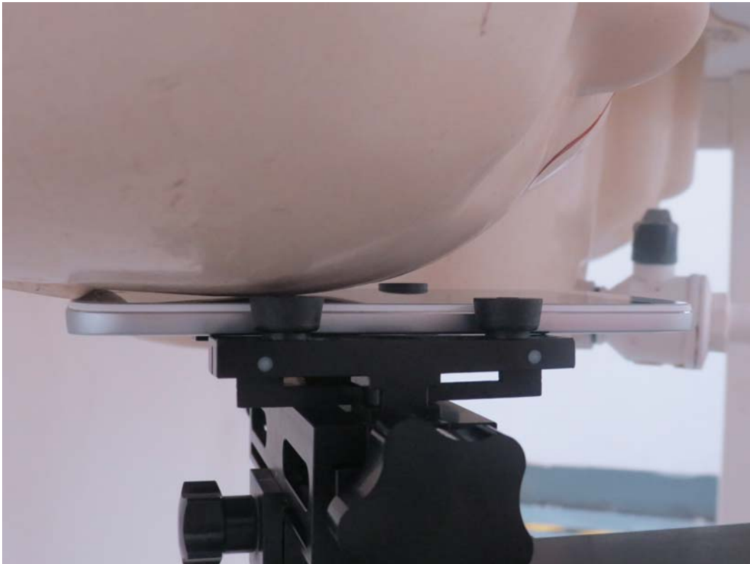
Picture 13: Right Hand Touch Cheek Position
