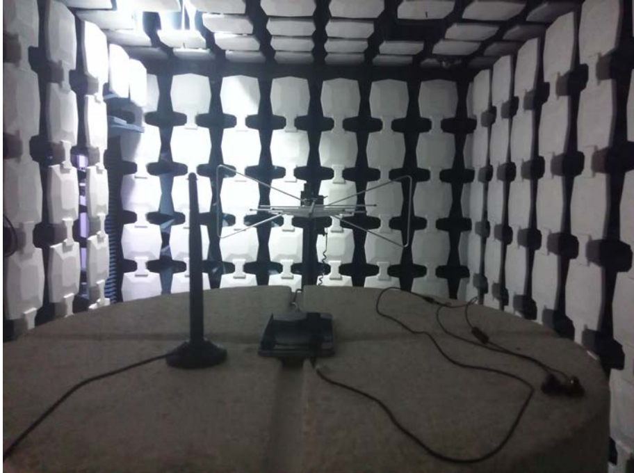
Radiated Spurious Emission (below 1GHz)
