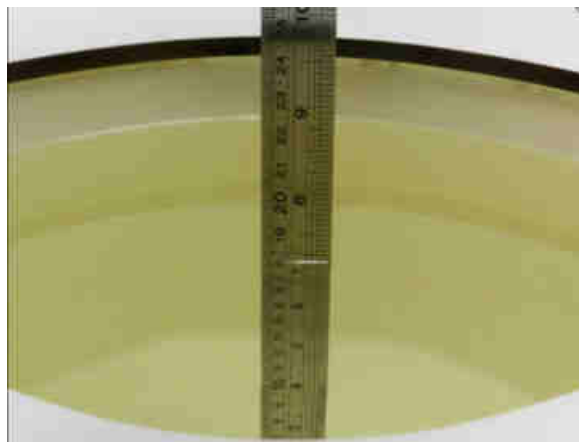
Fig 10.2 Photo of Liquid Height for Body SAR
