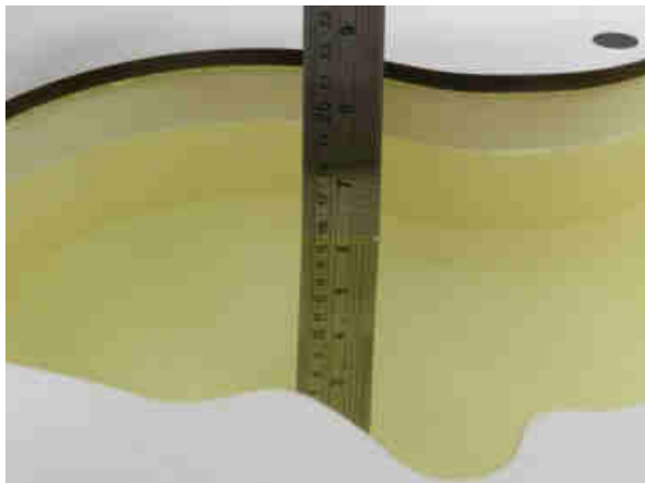
Fig 10.1 Photo of Liquid Height for Head SAR
