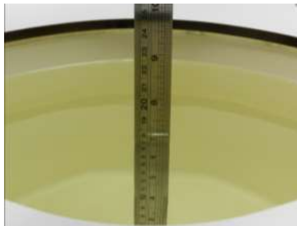
Fig 10.2 Photo of Liquid Height for Body SAR
