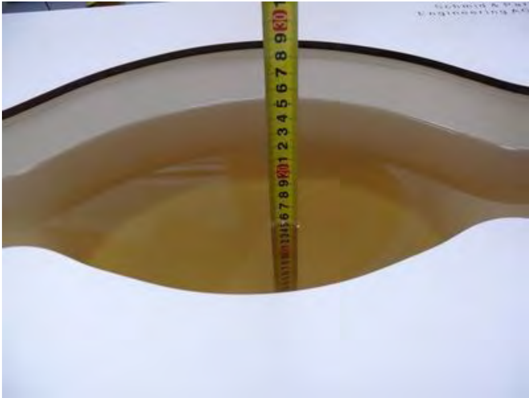
Picture 1: Liquid depth in the flat Phantom (750MHz, 15.4cm depth)
