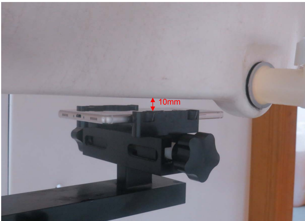
Picture 21: Front Side, the distance from handset to the bottom of the Phantom is 10mm
