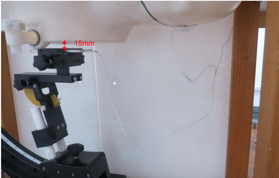
Picture 26: Back Side with Earphone, the distance from handset to the bottom of the Phantom is 15mm
