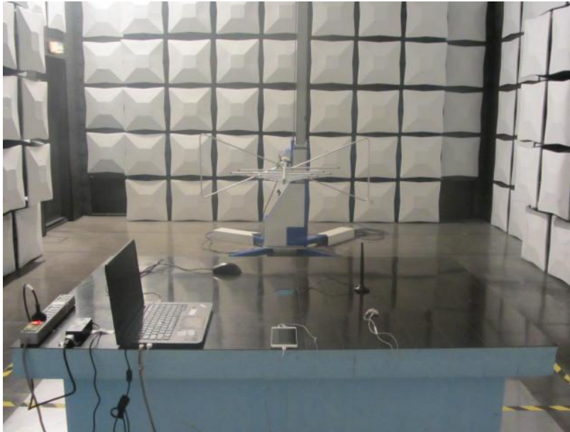
Radiated Spurious Emission (below 1GHz)
