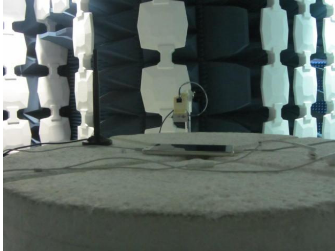
Radiated Spurious Emission (18GHz to26.5GHz)
