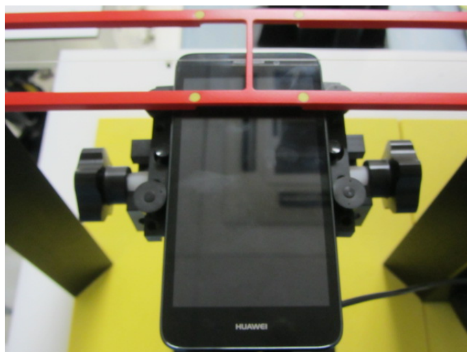
HAC T-coil test photo
