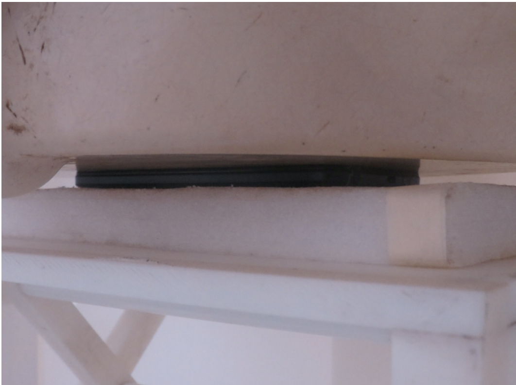
Picture 20: Front Side, the distance from handset to the bottom of the Phantom is 0mm
