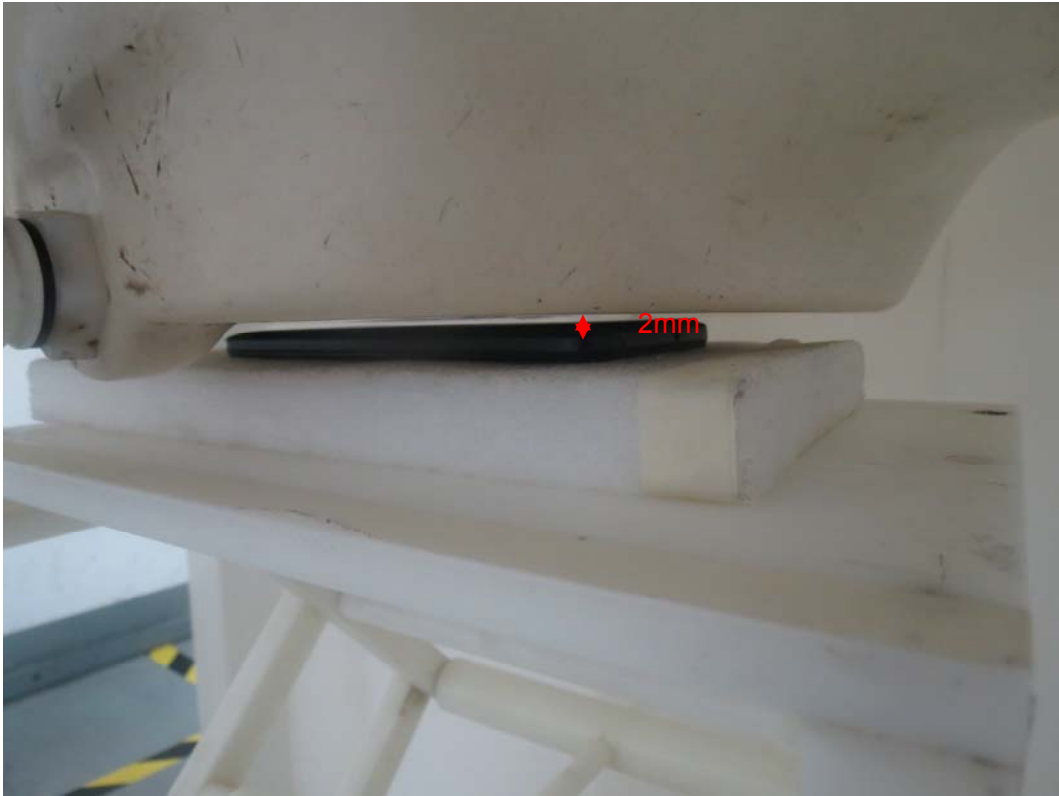
Picture 17: Back Side, the distance from handset to the bottom of the Phantom is 2mm
