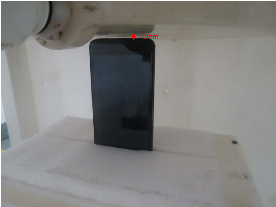
Picture 18: Bottom Edge, the distance from handset to the bottom of the Phantom is 2mm
