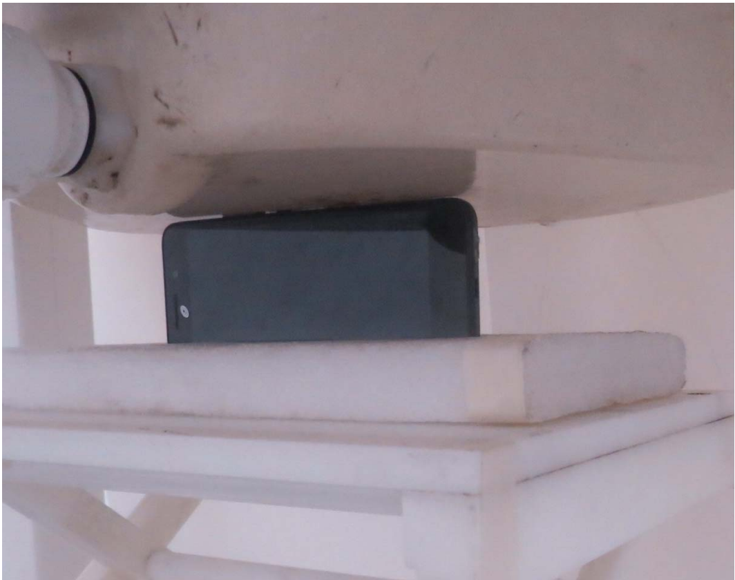
Picture 22: Right Edge, the distance from handset to the bottom of the Phantom is 0mm
