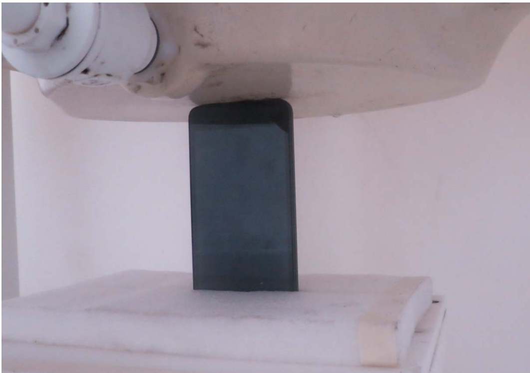
Picture 24: Bottom Edge, the distance from handset to the bottom of the Phantom is 0mm
