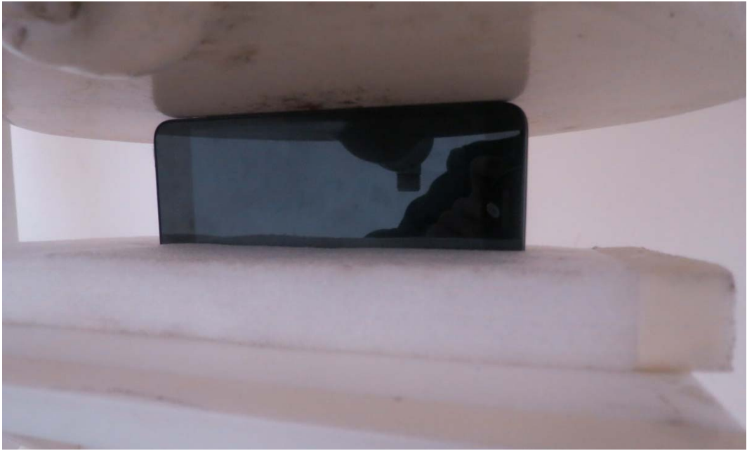
Picture 21: Left Edge, the distance from handset to the bottom of the Phantom is 0mm
