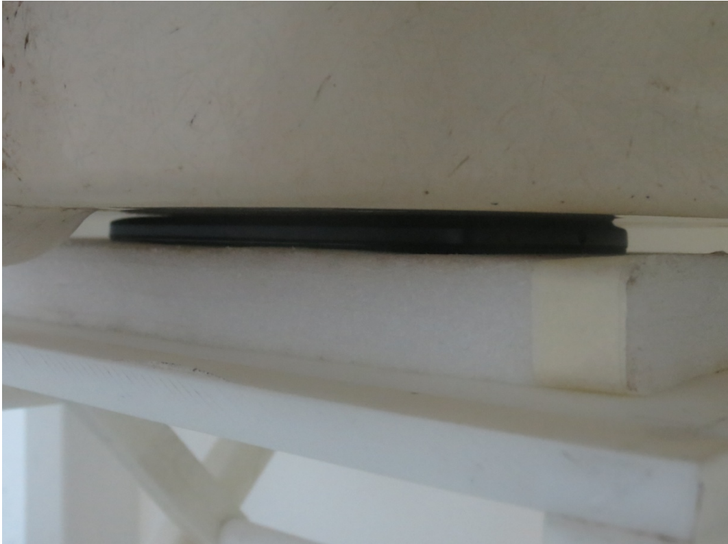
Picture 19: Back Side, the distance from handset to the bottom of the Phantom is 0mm
