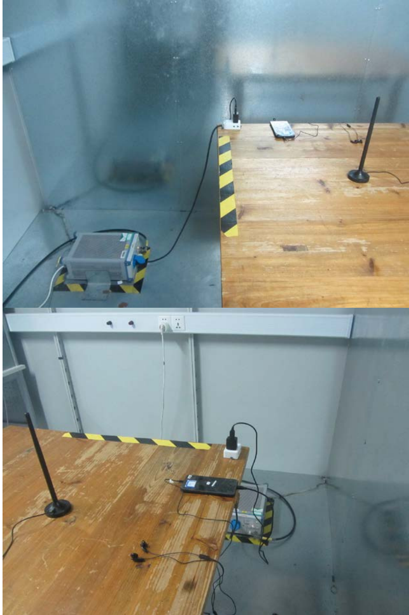
Conducted Emissions for AC Ports
