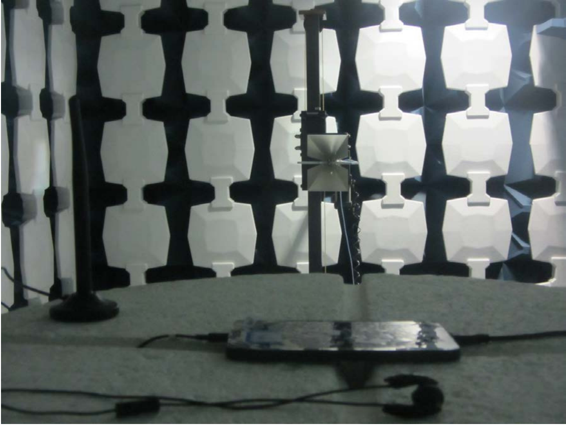
Radiated Spurious Emission (3GHz to18GHz)
