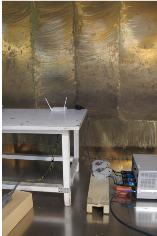
Conducted emissions of AC power port
