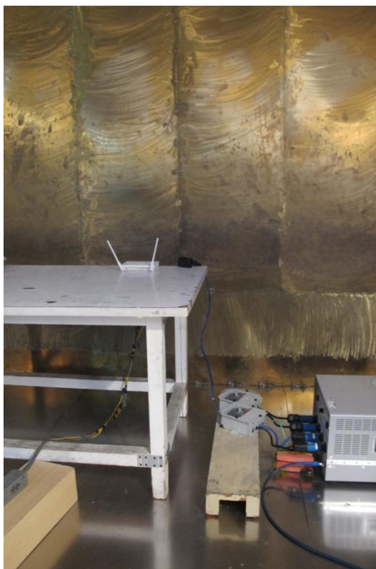
Conducted emissions of AC power port
