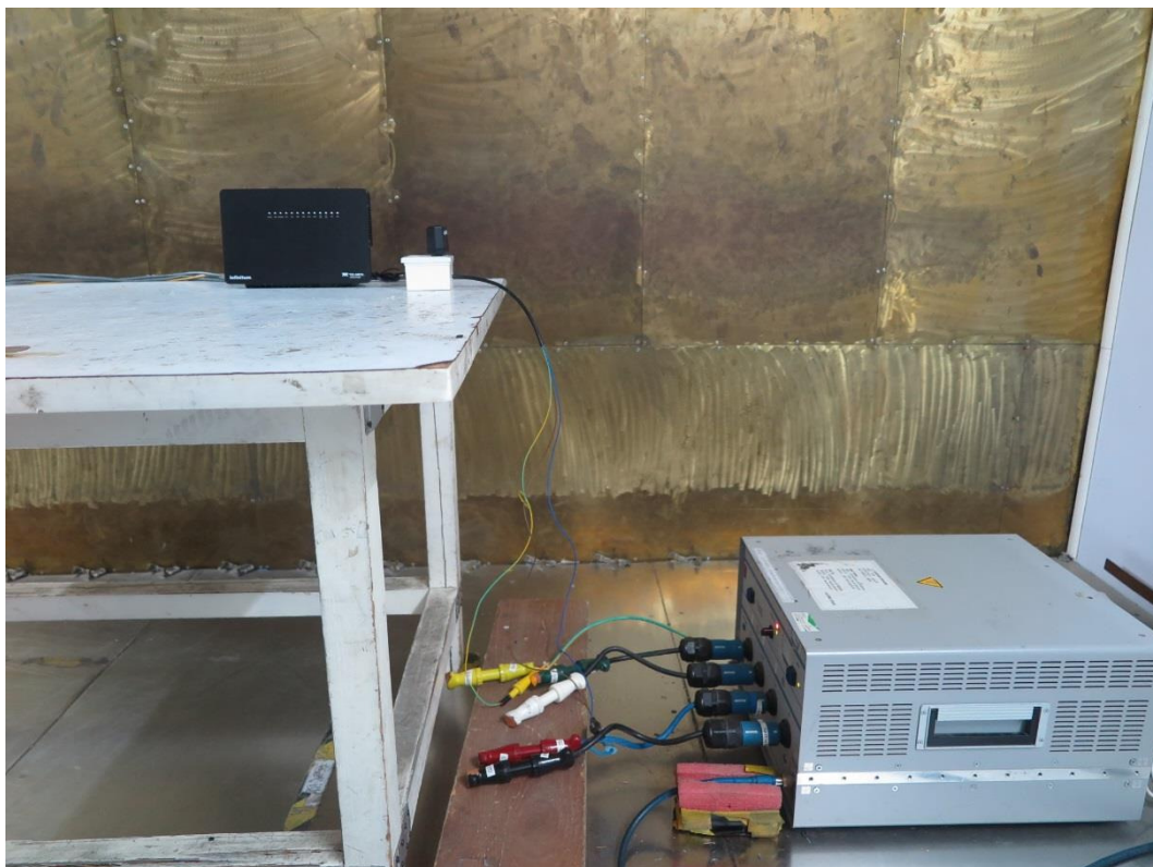
Conducted emissions of AC power port
