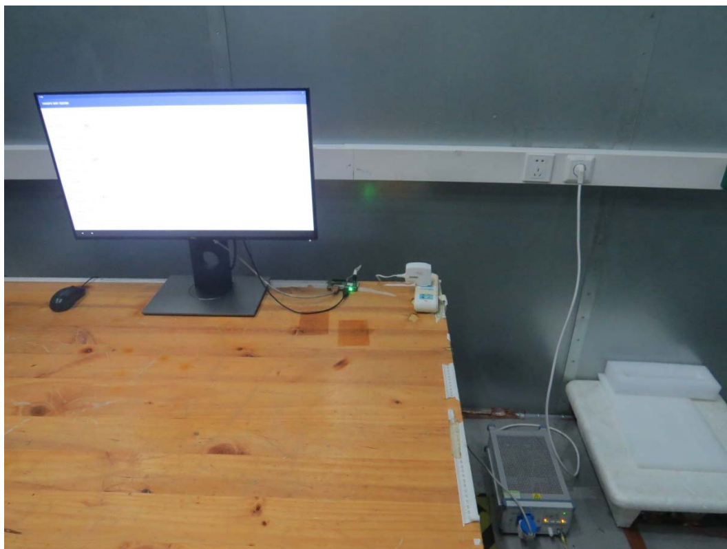
Picture 3 Conducted Emission Test Setup
