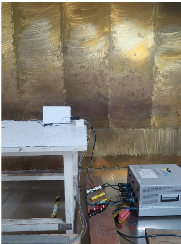
Conducted emissions of AC power port
