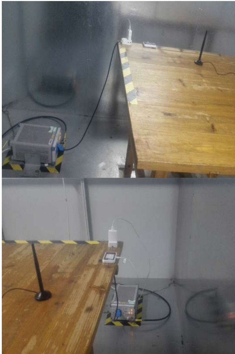
Conducted Emissions for AC Ports
