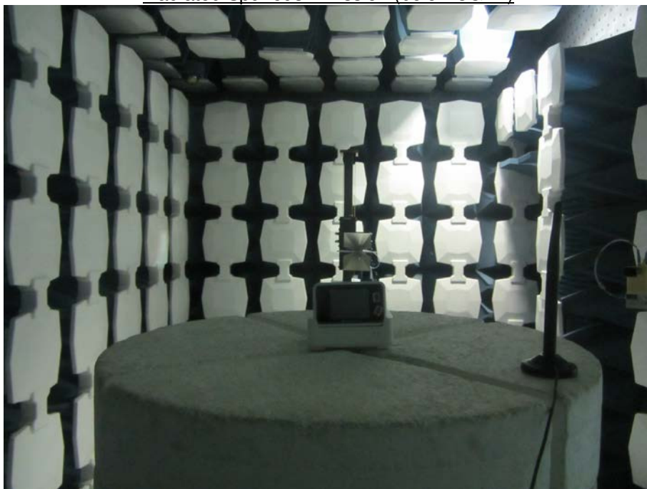
Radiated Spurious Emission (3GHz to 18GHz)
