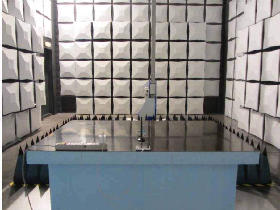
Radiated Spurious Emission (above 18GHz)
