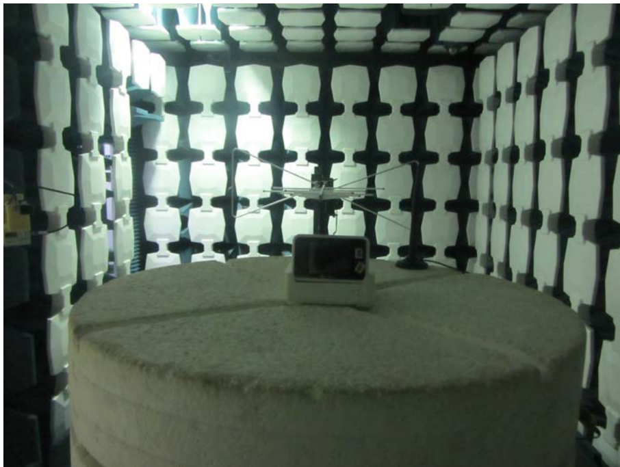
Radiated Spurious Emission (below 3GHz)
