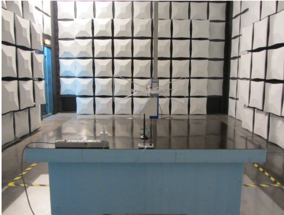
Radiated Spurious Emission (below 1GHz)
