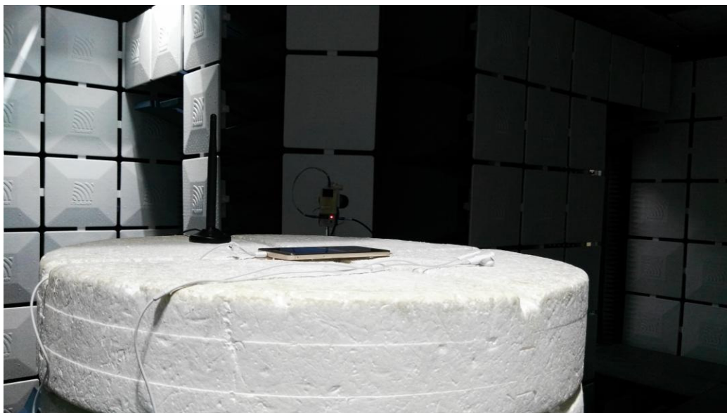
Radiated Spurious Emission (18GHz to26.5GHz)
