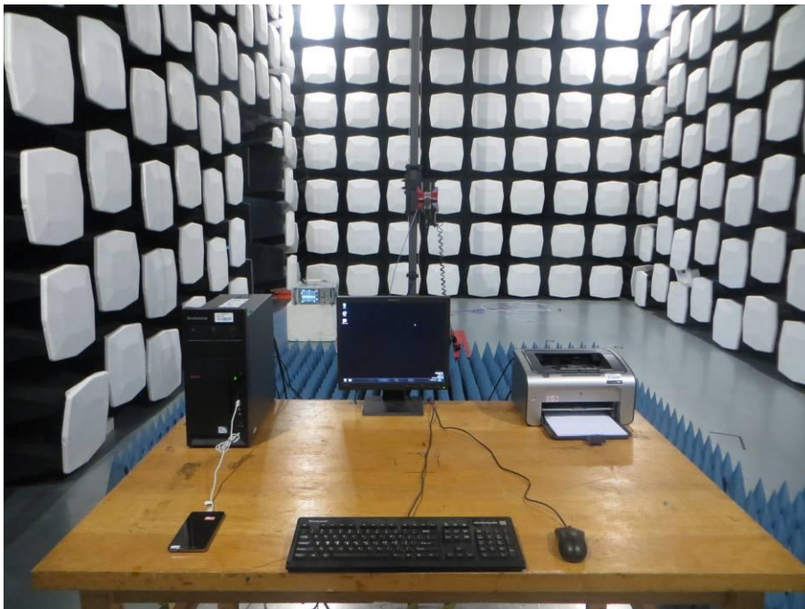
2. Radiated Emissions (Part 15B PC mode)(Above 1GHz)
