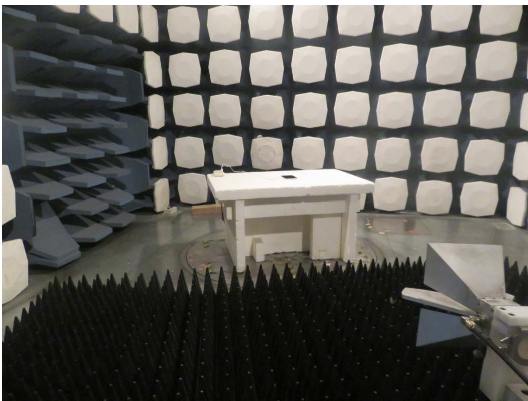
Picture 1: Radiated Spurious Emissions Test setup
