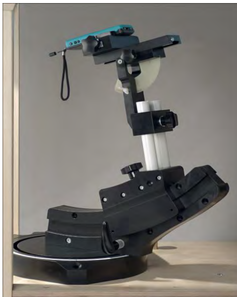
F-2. Device Holder for Transmitters
