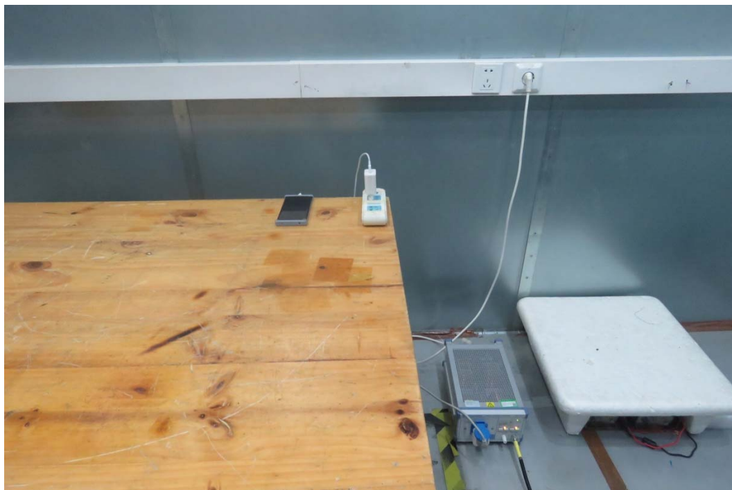
Picture 2 Conducted Emission Test Setup
