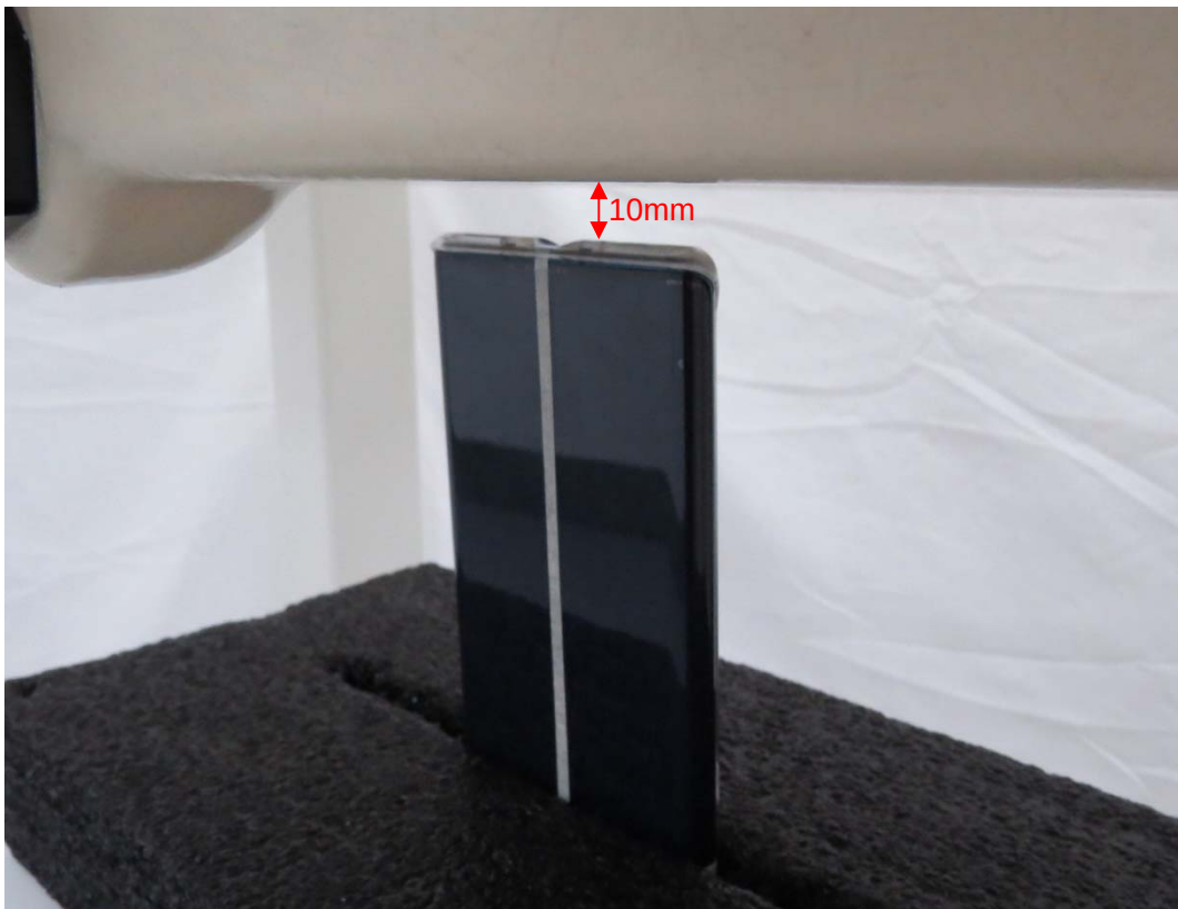
Picture 22: Bottom Side, the distance from handset to the bottom of the Phantom is 10mm (Mobile phone case (transparent))
